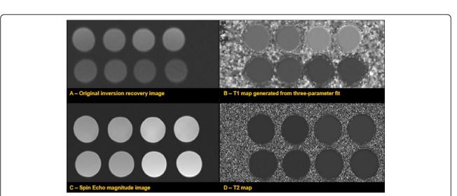
**Figure 1 T1 and T2 maps (B&D) generated from eight 11-cycle MOLLI images (A) and multiple TE spin-echo images (C)**. Two bottles of each tissue phantom were made because larger volumes of NiCl<sub>2</sub>-agarose gels improve composition accuracy. The bottles were averaged for T1 and T2 measurements.
