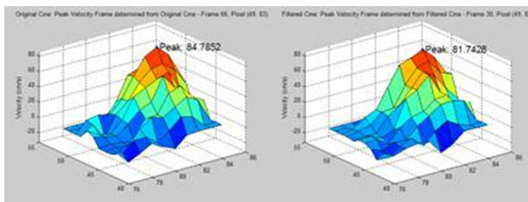
**Figure 1** Velocity profiles showing peak velocity measurement for original real-time cine (left) and KLT filtered cine (right).
