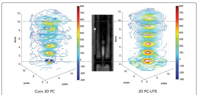
**Figure 1** Contour plots of the through-plane velocity in the jet after the 3 mm stenosis. The 3D PC-UTE sequence has less artefacts and measures a higher peak velocity than the conventional sequence.
