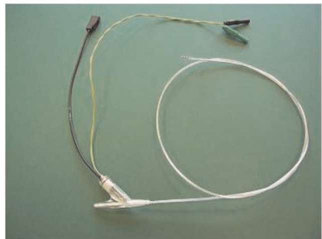
Diagnostic RF-safe MR-EP catheter.
