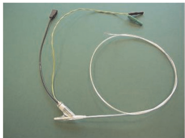
Diagnostic RF-safe MR-EP catheter.
