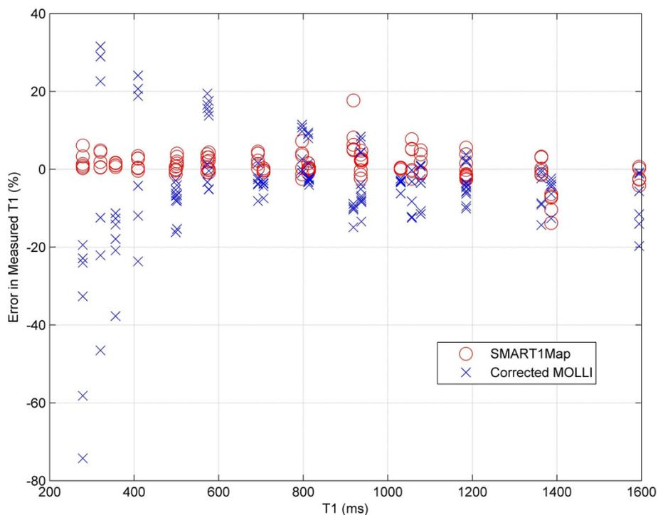
**Figure 1** Percent error in measured T1 for all experiments from SMART<sub>1</sub>Map and MOLLI compared with reference T1 from IR spin-echo. The significantly higher errors for MOLLI at lower T1s could be problematic for post-contrast-enhanced imaging, where T1s are expected to be less than 500 ms.
