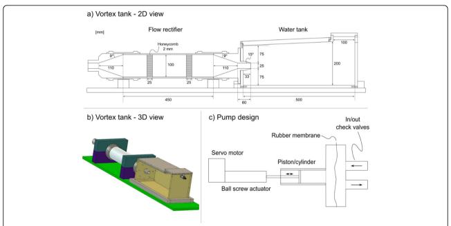
**Figure 1 Design and construction of the vortex ring flow phantom.** a) 2D view of the flow rectifier and vortex ring tank. All measures are in millimeters (mm). b) 3D view of the flow rectifier and vortex ring tank. c) Pump design. A servo motor powers a ball screw linear actuator, which in turn moves a piston-cylinder apparatus. A rubber membrane separates the flow medium from the pump to prevent abrasive particles from entering the piston/cylinder apparatus.
