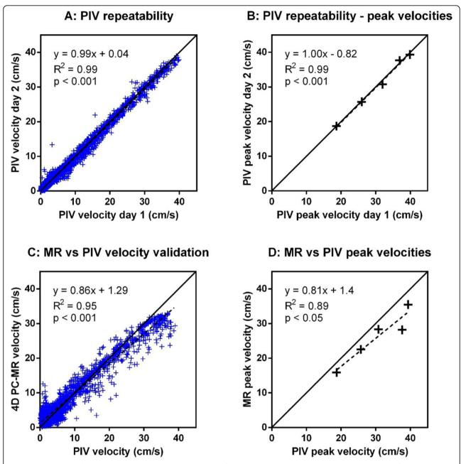
**Figure 2 Experimental results.** Panel A: Pixel-wise PIV repeatability for the highest pump setting. Panel B: PIV repeatability for peak velocities for all five pump settings. Panel C: Validation of 4D PC-MR velocities against PIV for the highest pump setting. Panel D: Validation of 4D PC-MR peak velocities against PIV for all five pump settings. 4D PC-MR underestimated peak velocities by 8-25% compared to PIV. All data taken at 400 ms from the initiation of flow.
