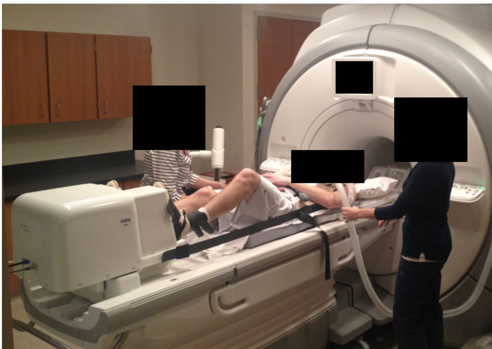
Fig. 1 Sample setup for exercise imaging. The subject lies in a supine position and steps against the pneumatic pedals of the cardiovascular magnetic resonance (CMR)-compatible exercise stepper (seen at the end of the CMR bed). The pressure supplied to the pedals control resistance. The subject is connected to the stepper with Velcro straps around the feet and a harness around the chest to minimize bulk motion during exercise
