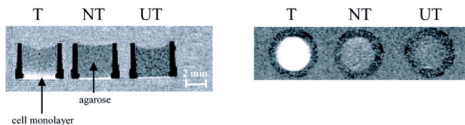
Figure 4 Molecular imaging of tissue factor expression on cultured smooth muscle cells. Cell cultures were incubated with tissue factor targeted nanoparticles (T), nontargeted nanoparticles (NT) or no nanoparticles (UT). Left: Spin-echo images of smooth muscle cell monolayers acquired at 1.5T reveal image enhancement for the well treated with targeted particles, but not the wells receiving nontargeted or no nanoparticles. Right: A maximum intensity projection through the 3 D stack of T1-weighted images acquired parallel to the cell monolayers demonstrates the sensitivity of this targeting method for detecting labeled cells. Reprinted with permission from Morawski, et al [74].
