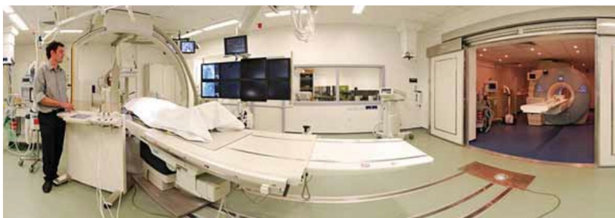
Figure 9 Hybrid CMR/cardiac catheterization laboratory. Fish-eye view of a hybrid CMR/cardiac catheterization lab - The bi-plane catheter lab (left) is connected to the MR scanner room (right), via a set of sliding doors (open). The pedestal of the catheter table slides toward the MR scanning room to join with the MR scanner table. The patient then slides across between the two tabletops, using Miyabi table technology (Siemens AG).
