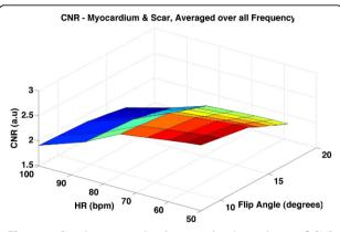
**Figure 1** Simulations results showing the dependence of CNR between mycardium and scar on HR and flip angle.
